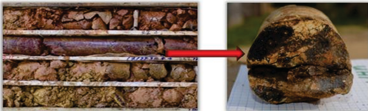
Fig. 6. Crushed stone with sandy loam aggregate in the Lithomarge zone
