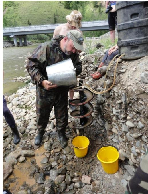
**Figure 4.** Dr. Vladimir Naumov is demonstrating the sluicing apparatus used to separate the heavy mineral and clay fractions in the field (Beliy Ius River). The principle behind the technique is that grains are separated in the sluice owing to their density
