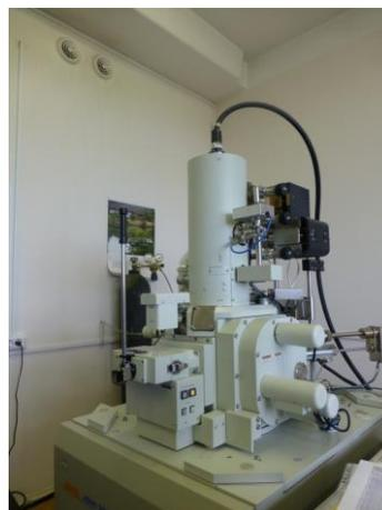
**Figure 6.** The JEOL JSM-7500 Field Emission Scanning Electron Microscope at Perm State University used to examine and image gold particles
